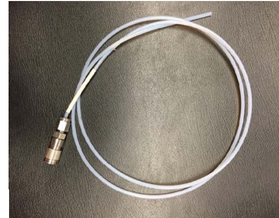
Capillary Flow Controller (0.10mL/min & 0.31 mL/min)
