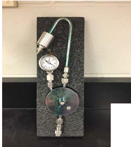
Diaphragm Flow Controller (3.0 mL/min)
